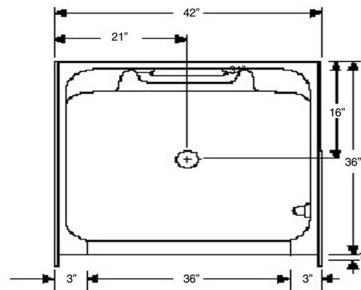
Galvanized steel reinforced and/or wood reinforcement will vary due to application of accessories
