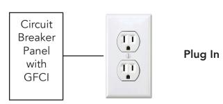
120 Volt, GFCI circuit, minimum 5 amps per control
