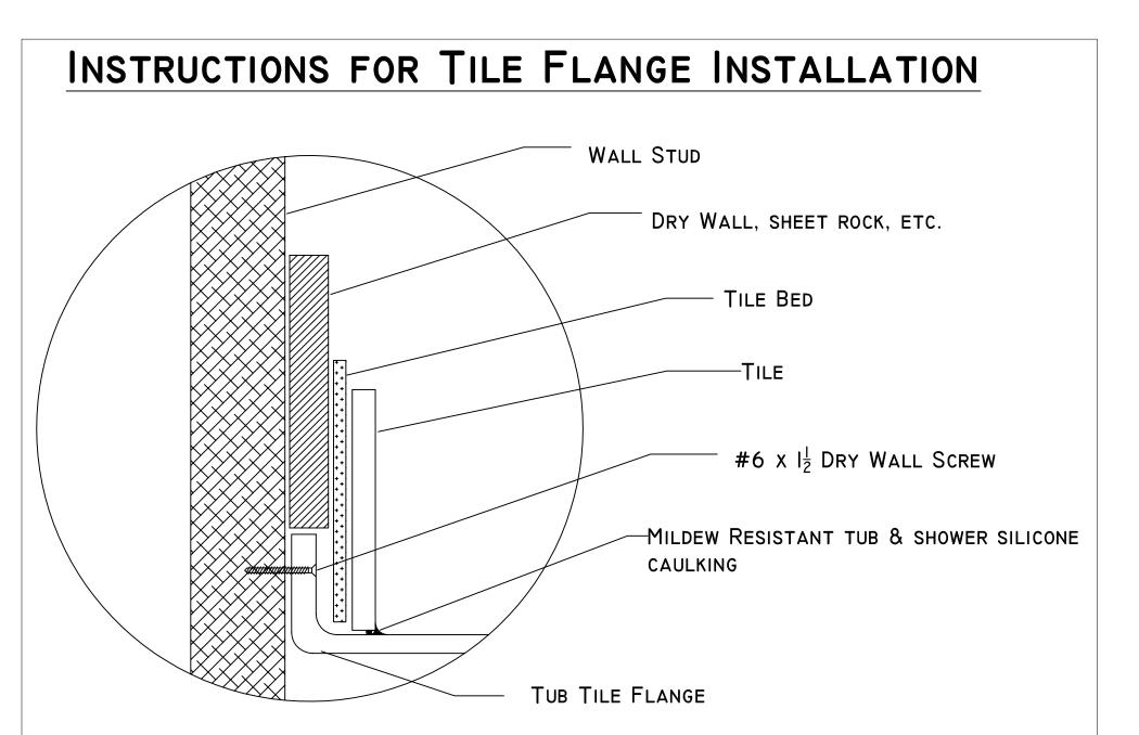
IMPORTANT NOTE: PRE-DRILL HOLE INTO TUB TILE FLANGE BEFORE INSTALLING SCREW. DO NOT CINCH OR TIGHTEN TILE FLANGE TO STUDS. THIS CAN CAUSE FLEX IN THE UNIT THAT MAY CAUSE THE DOOR TO LEAK.
