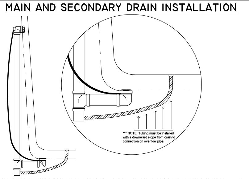
THE DRAIN HOSE MUST BE INSTALLED WITH NO KINKS OR SHARP BENDS. THE PROVIDED FITTING WITH BRASS BARB MUST BE INSTALLED AT THE LOWEST POINT POSSIBLE OF THE OVERFLOW PIPING, BELOW THE SANITARY T, ALLOWING THE MAXIMUM SLOPE FOR DRAINIAGE FROM THE SECONDARY DRAIN TO THE OVERFLOW.
